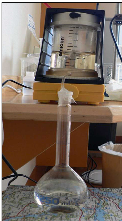
Photo 3. Frontal ultrafiltration was performed with a 400 mL polycarbonate cell (Amicon 8400) with a suspended magnet stirring bar located above the filter in order to prevent clogging during ultrafiltration. Nitrogen pressure (around 2.5 bars) was used as the driving force, and a concentration factor of 6 was applied (For more details see in Cheryan, 1998).
