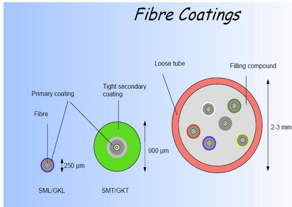
Figure 1 Fiber coatings, tight buffer and loose tube. [4]
