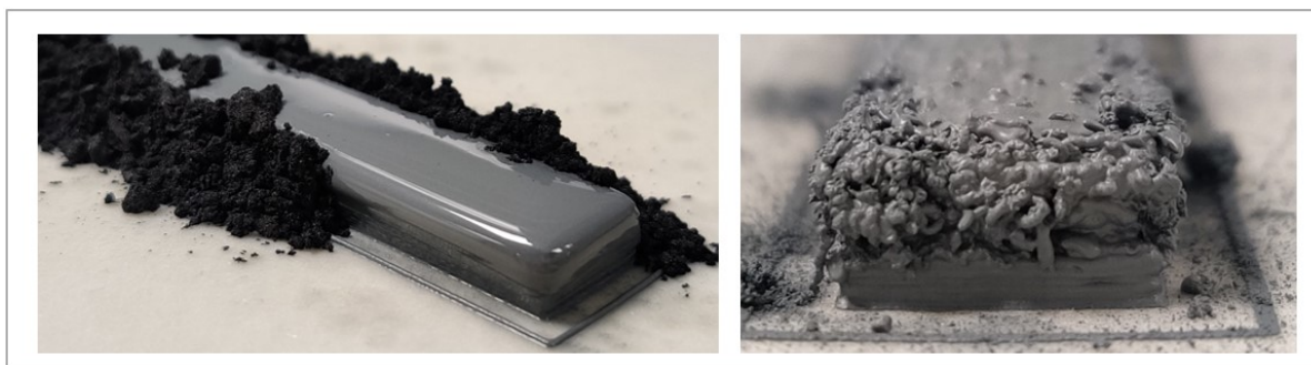
Figure 30 The assumed separation behavior in AOT-containing inorganic pastes. The first bar of the same batch (left) seemingly contained a larger concentration of oil than the second bar (right).
