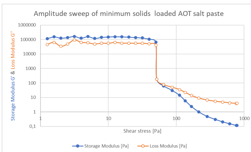
Figure 23 Amplitude sweep of minimum solids loaded salt paste with 2.5 wt-% AOT.
