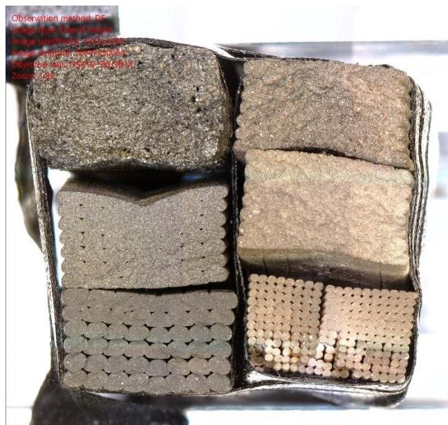
Figure 42 Crosscuts of IO1 (left) & IO2 (right) bars containing different sized particles. Desired particle sizes from top to bottom: 80, 280, 1000.
