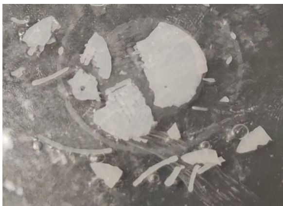
Figure 29 Salt structures shattered when attempted to freeze them with liquid nitrogen.
