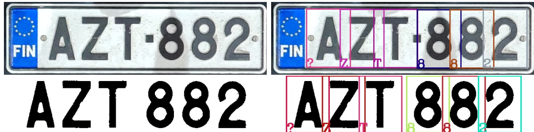
Figure 56: Template matching with and without cleaning, the "?" character recognized was the Swedish letter "Å", in both cases, otherwise all matches were correct.
