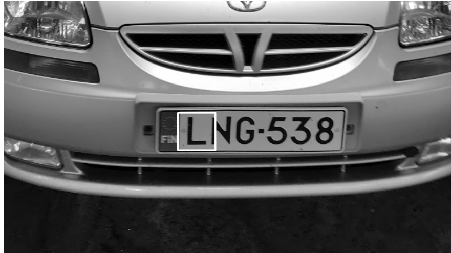
Figure 54: The template matching algorithm was used to search for the letter L using a template created from using the din1451mittelschrift font (seems to be one of the closest, free alternatives, to the Finnish license plate font). Each available method was run 100 times and the average execution time was calculated: around 5ms. The image used is of the dimensions 768 \times 432 . "TM_CCOEFF" was the fastest of the ones that was positioned correctly.
