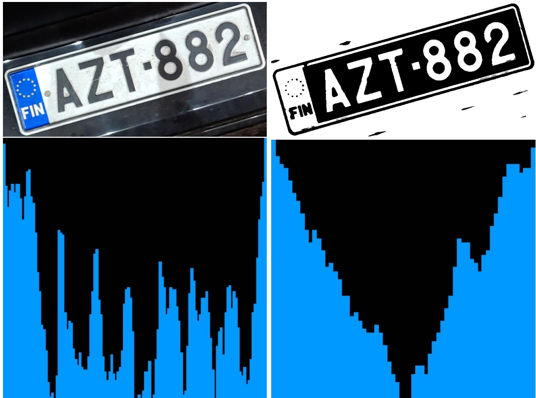
Figure 51: The original image, the cleaned and thresholded image, the pixel intensity by column and the pixel intensity by row.
