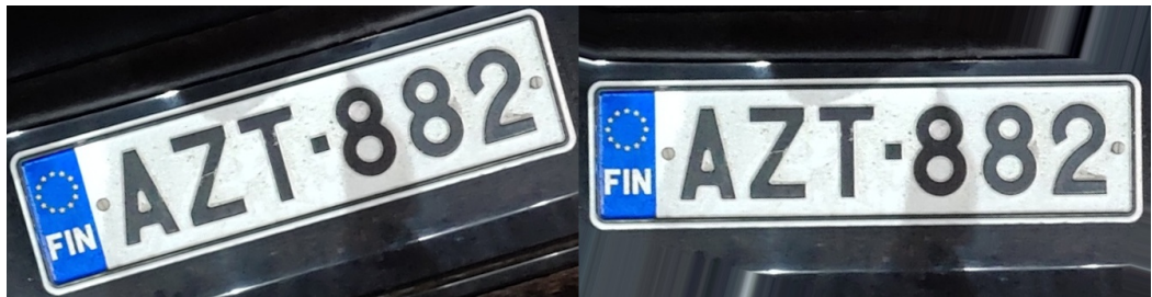
Figure 26: Simple skew correction of license plate. Processing time 16ms. Testing angles -15 to +15.
