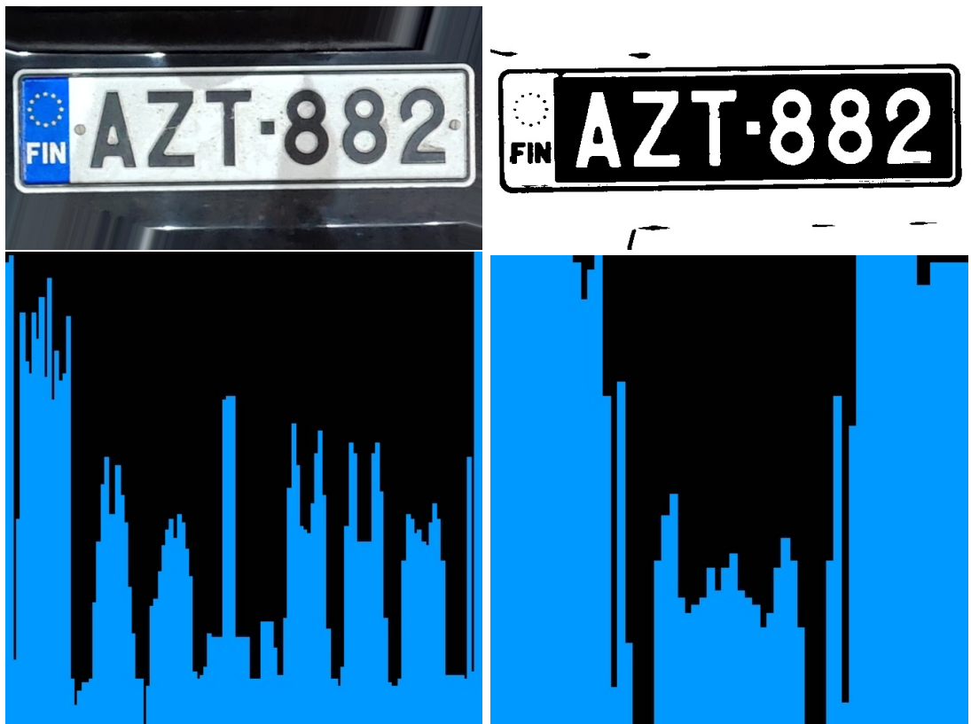
Figure 52: The original image, the cleaned and thresholded image, the pixel intensity by column, the pixel intensity by row.
