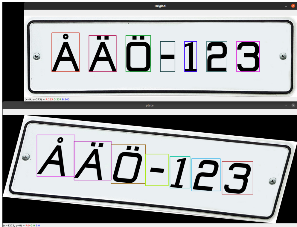
Figure 38: The bounding boxes of a license plate need to be adjusted after perspective transform.
