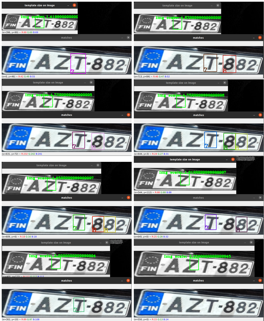
Figure 59: Comparison of matches found depending on the size of the template relative to the license plate image. The first match was found when the image height was 1.42 times the template height, and no matches were found starting from 2.6 times the template height.
