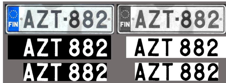
Figure 48: Image variants of AZT-882 license plate that Tesseract OCR was tested on. The original image was of size 650 \times 180 and the others were the same or smaller. The processing time varied between 100ms and 140ms.
