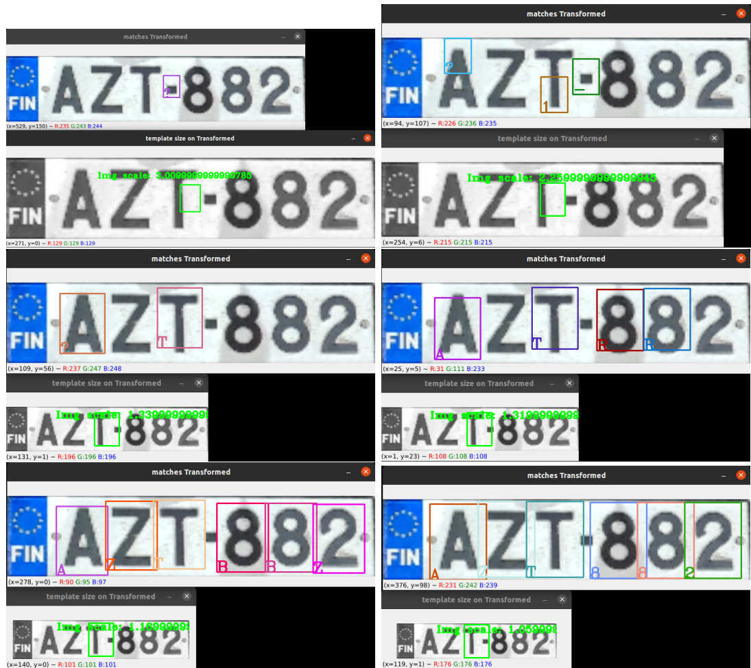
Figure 60: Comparison of matches found depending on the size of the template relative to the license plate image on a perspective corrected image at a few different values of scale. Going down to a 1 to 1 plate-height to template image-height yields the best (perfect) results, which makes sense, as the template images were generated with the same padding as is used in the Finnish license plates and the transformed image license plate is cropped (nearly) perfectly.
