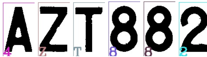
Figure 57: Template matching on individual character crops. Total processing time: 6.4ms. Templates: 40. Template size: 32×24. Image size: 32×24. Looking at the "A" character crop compared to the "A" template, the bottom right "intersection" matches that in the "4" template better than the "A" template.
