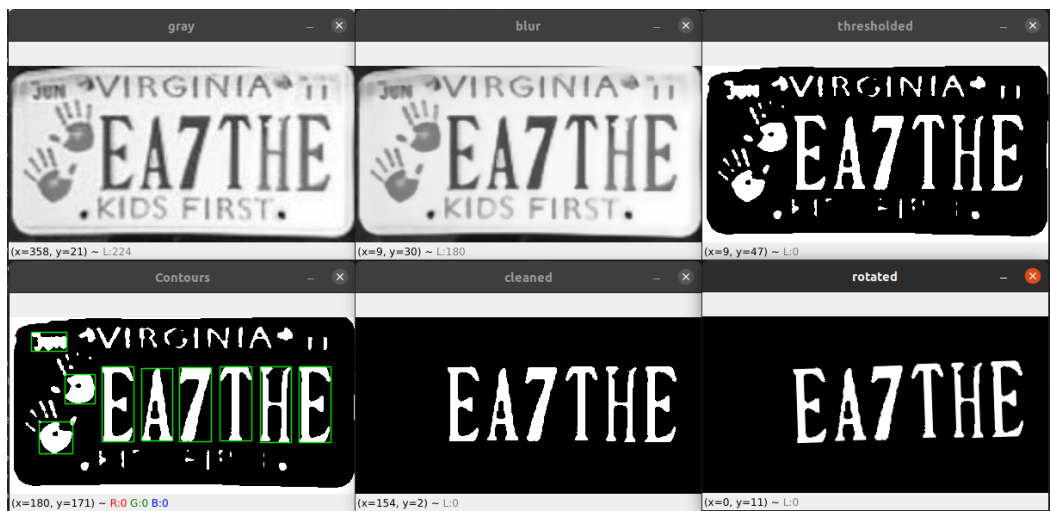
Figure 63: The cleaning process of an image before passing it to Tesseract OCR. The "cleaned" image was the final result, in which Tesseract OCR correctly found the text "EA7THE", however, the "rotated" image was intentionally rotated by 2 degrees and after which Tesseract OCR recognized "Vail" instead.
