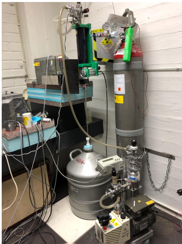
Figure 3.3: Cryostat and dewar for liquid N 2 .
