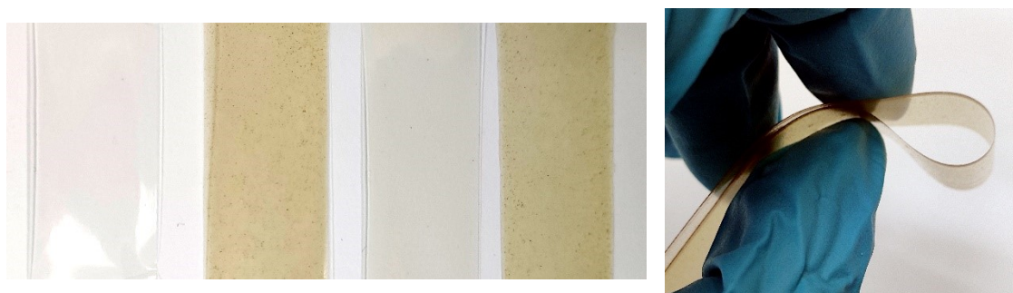
Figure 7. Films with glycerol as a plasticizer. From left: unloaded film, unloaded film with liver powder, drug-loaded film, and drug-loaded film with liver powder. Right: a drug-loaded film with liver powder.
