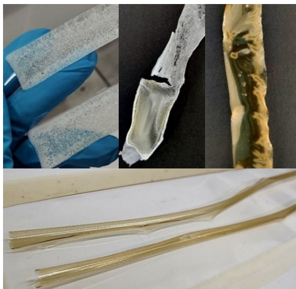
Figure 6. Upper pictures: gabapentin crystallized in the cast films obtained from 5% drug-loaded solutions. Lower picture: the films with polyethylene glycol 400 as a plasticizer hardened and curled up when drying in ambient conditions.
