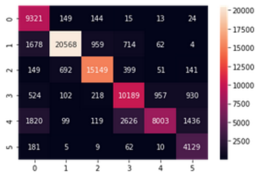
Figure C.1: The confusion matrix of the predictions for the separated training set. The diagonal shows the correct predictions of the models, wrong predictions are the surrounding area. The values within the cells are the number of predictions for the class. The model can generalize well to the separated training set.
