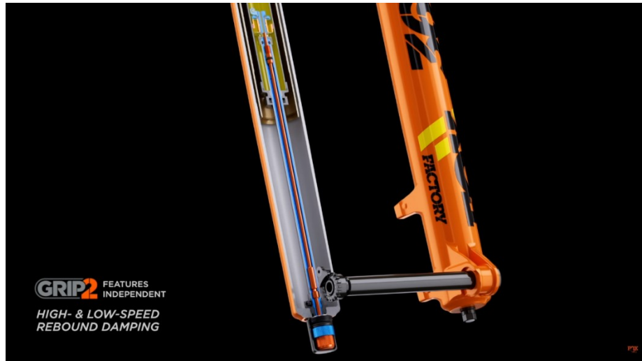
Figure 4: Grip 2 LSR-HSR adjustment, © Fox Racing Shox
