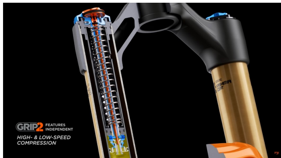
Figure 3: Grip 2 LSC-HSC adjustment, © Fox Racing Shox
