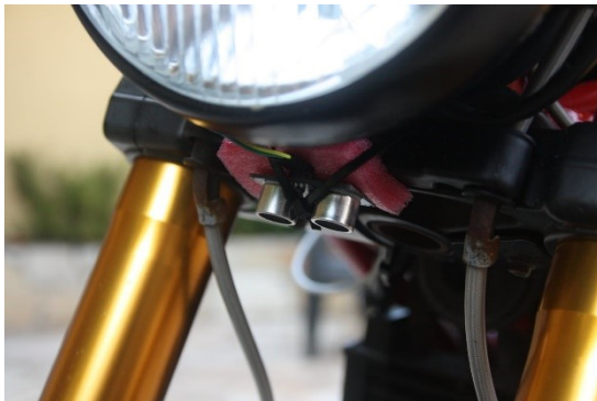
Figure 14: Ultrasonic sensor fork mount, © D. Longo
