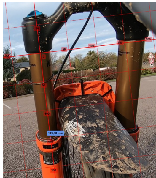
Figure 53: Kinovea coordinate system and calibration
