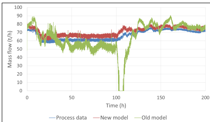
Figure 43. Test result for the suction mass flow of the normal operation case using the ideal equation of state.
