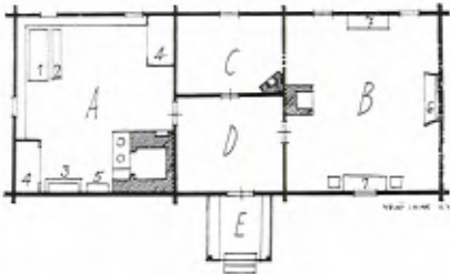
45. Twin room cabin. A. tupa (multi-purpose main room), B. sali ("parlour"), C. porstokamari (backchamber), D. porsto (entrance-hall passage), E. pislakki (porch). Measurement drawing MV. Photo SRM.
