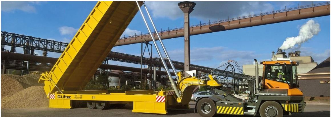
Image 2: A special cassette with lift for industrial use (source: NT Liftec OY)
