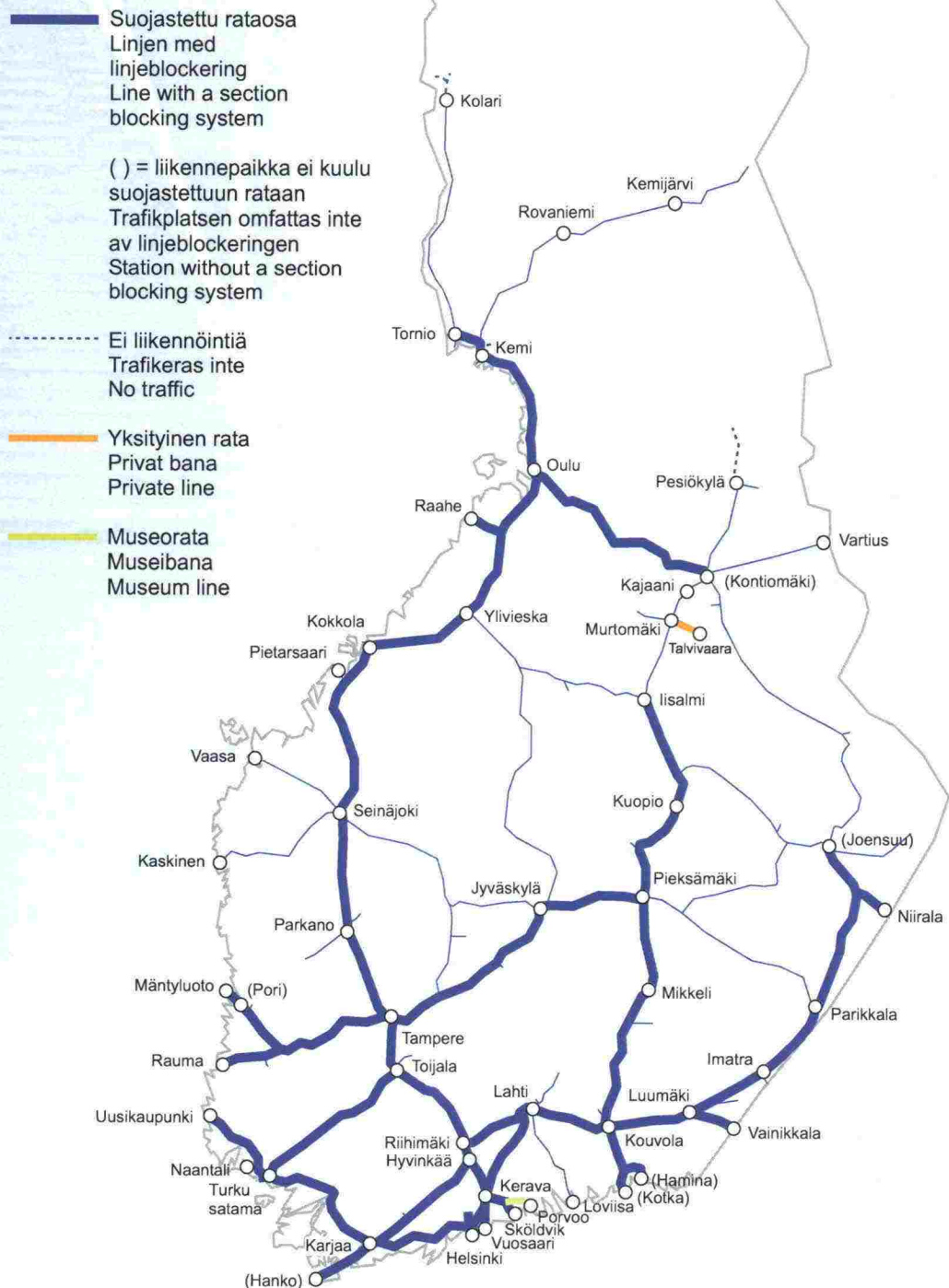
Figure 1. Lines with a section blocking system.
