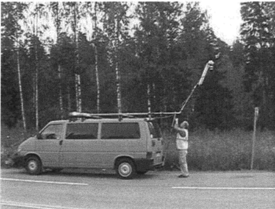
Figure 11. Crack measuring device, The Finnish Road Enterprise, version 2004
