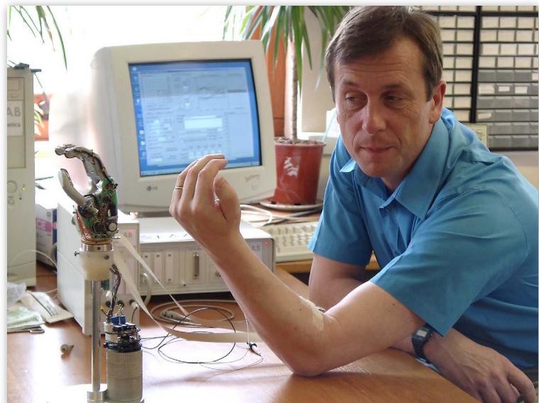
Robot hand controlled by (author's) neural signs.
