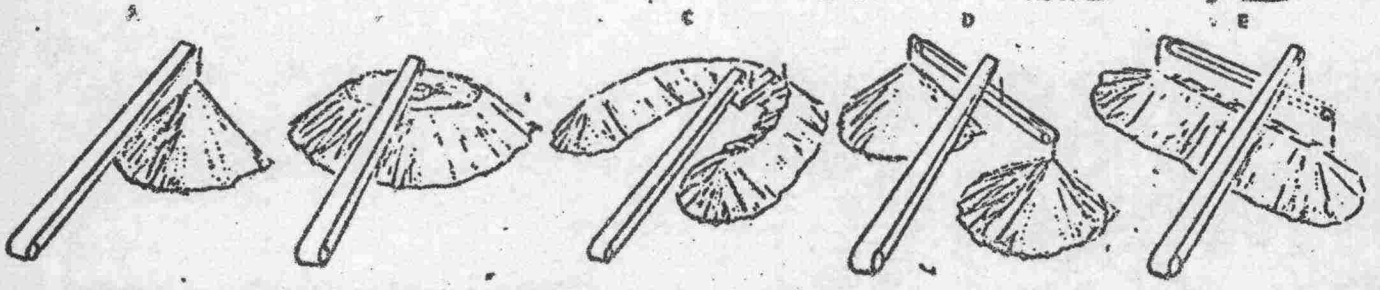
Single stationary conveyers (from left to right): (A) no auxiliary—conical pile; (B) with slinger—conical pile; (C) with pivoted boom—radial windrow; (D) with reversible belt—two conical piles; (E) with shuttle belt—windrow
