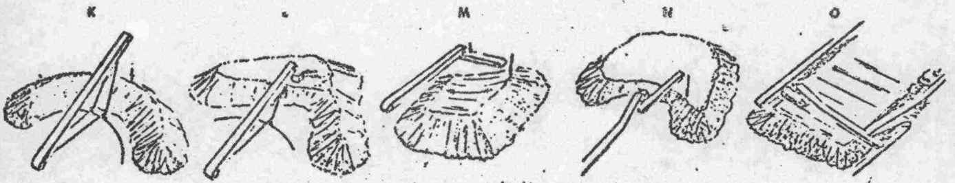
Conveyors (from left to right): (K) radial stacker, no auxiliary—radial windrow; (L) radial stacker, with slinger or thrower—radial windrow; (M) stacker, with radial boom—windrow; (N) stacker, with traveling radial boom—windrow; (O) bridge conveyor, with tripper—windrow
