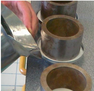
Figure 4. Pouring wax on the cartonboard edges for WVTR determination.
