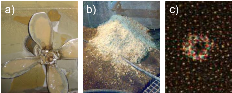
Figure 2.1 Examples of calcium oxalate scale problems: a) hard layers of scale on machine chest wall; b) crumbled scale particles from the bottom of the machine chest that could follow the pulp stream and end up in the paper; c) print defect (“hickie”) caused by calcium oxalate particle.
