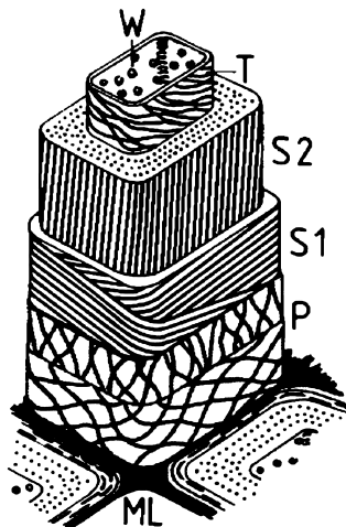
Figure 1. Model of the cell wall structure of softwood tracheids and hardwood libriform cells. ML: middle lamella (0.1–1 \mu\text{m} ), P: primary wall (0.1–0.3 \mu\text{m} ), S 1 : outer secondary wall (0.1–0.2 \mu\text{m} ), S 2 : secondary wall (1–5 \mu\text{m} ), T: tertiary wall or inner secondary wall (S 3 ) (0.1 \mu\text{m} ), W: warty layer (Fengel 1989).
