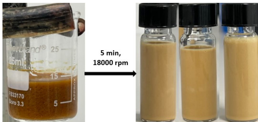
Figure 11. A stable looking emulsion before homogenisation, with three examples of homogenised emulsions. From the left: TSI 1.47 (1.2 g HLB 8), TSI 2.27 (1 g HLB 9), and TSI 1.60 (1.6 g HLB 8).
