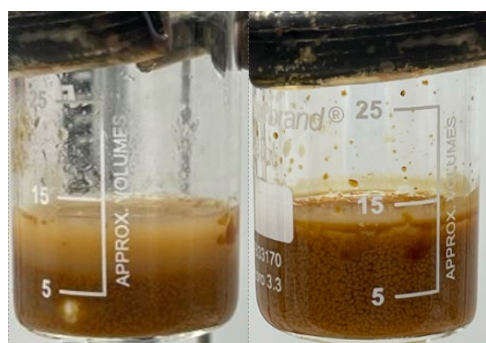
Figure 13. Two emulsions before the homogenising step. From the left: TSI 1.75 (1.4 g, HLB 9), TSI 3.60 (1.4 g, HLB 7).
