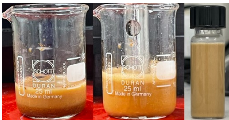
Figure 19. The different stages of a suberin emulsion with GGM-FA as surfactant. From the left: the emulsion before using the homogeniser, the emulsion while being homogenised, and the emulsion after being transferred to the vial.
