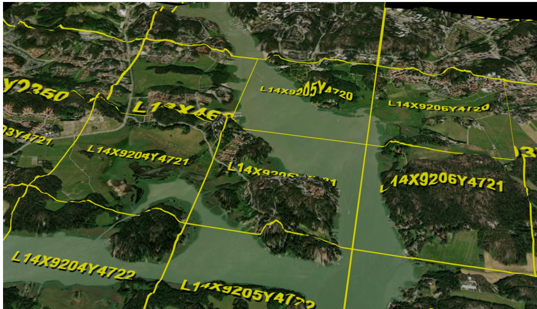
Figure 14. Interpolating points that appear on the edge of the tile. Tiles displayed in Cesium (height exaggerated by factor of 10).
