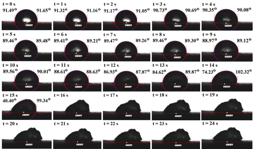
Figure S9. Temporal changes of the contact angle of GG in 24 seconds
