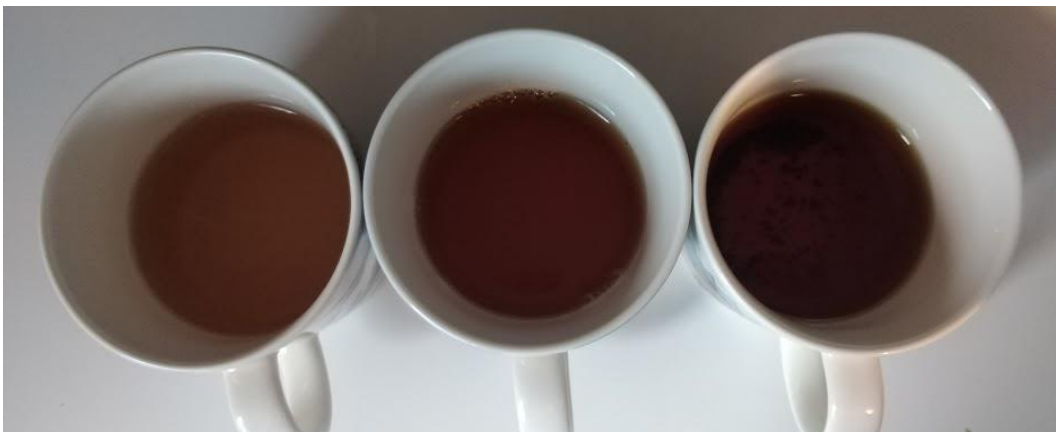
Figure 64. An example of how concentration of chemical in the solvent affects to the absorbance of light, pictured are tea concentrates at different levels of dilution with water from weakest to strongest (left to right) in which the thickness of the liquid is kept constant.
