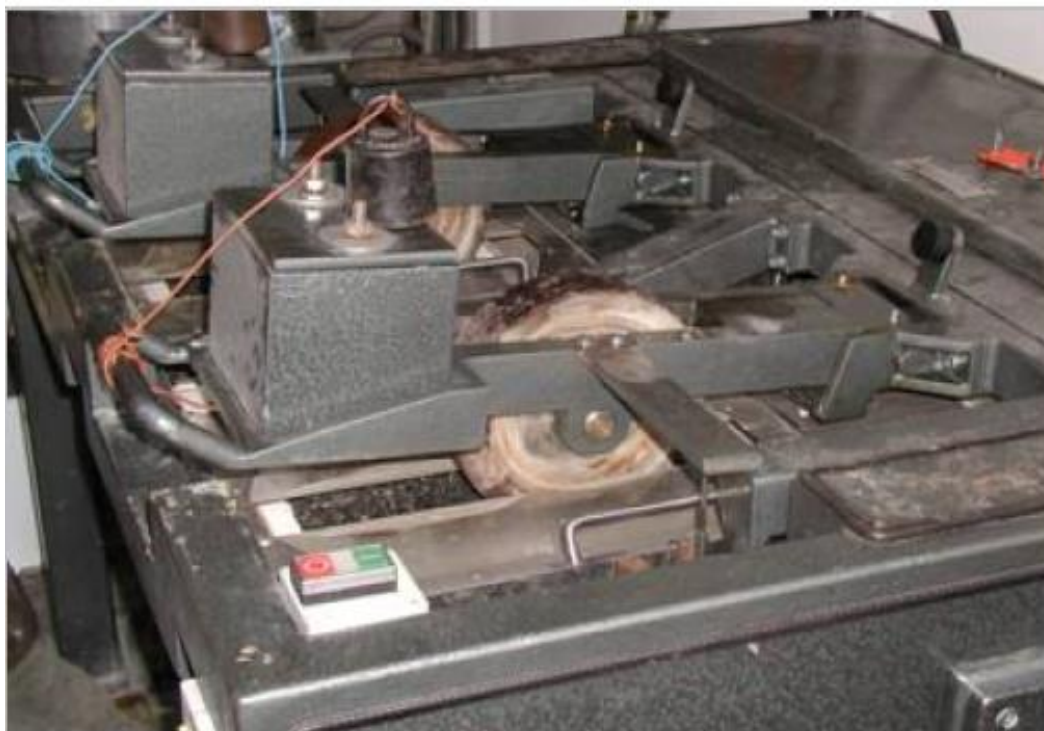
Figure 171. The Hamburg Wheel-tracking device (Olsson, Krona & Nordgren 2010).
