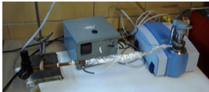
Figure 74. The picture of the setup used for in-situ aging by the method called ATRAC (Yut, Bernier & Zofka 2012).
