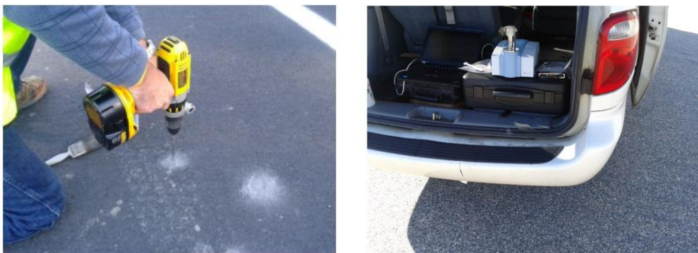
Figure 95. The ATR equipment can be portable and thus available for studies of roads in field, where a material is drilled into the form of powder and measured (Chrysochoou, Johnston & Yut 2014).
