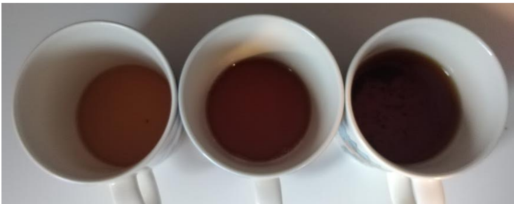
Figure 65. An example of how thickness of solution affects absorbance of light, pictured are tea concentrates of equal strength, where from left to right approximately 5 mm, 20 mm and 40 mm thick film is poured.
