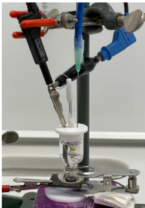
Figure 14: The small-scale configuration used to conduct the CV on the glassy carbon electrodes.
