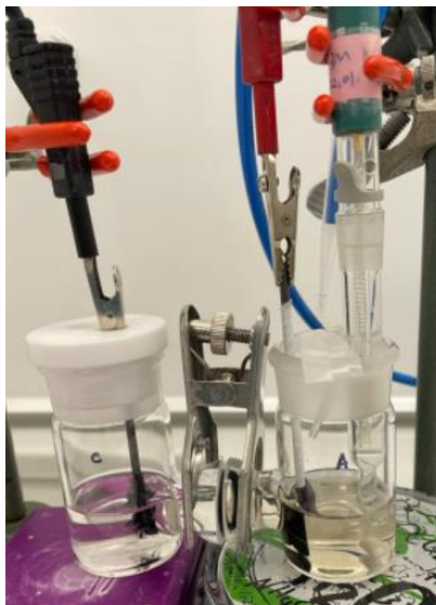
Figure 7: Image of the H-Cell set up used for the CV and chronoamperometric measurements.
