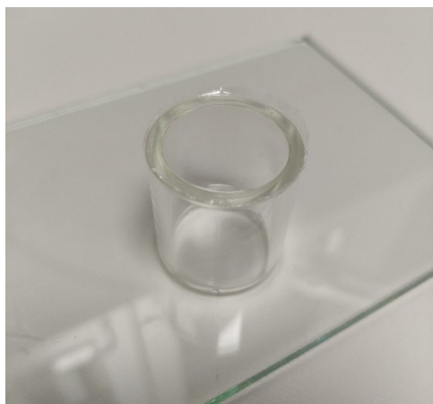
Figure 2. Set-up for membrane preparation.
