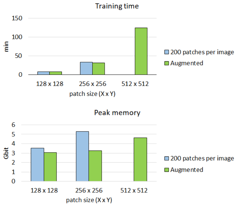
Figure 29. Training time increases little when patch size is higher. The real issue is memory usage and peak memory increases rapidly as patch size increases. Augmented data (20 images augmented to 630 images, the green bar) consumes less memory than patches (20 images - > 4200 patches, the blue bar). Memory limit exceeded when patch size was 512 x 512 pixels and patches were used. The training parameters in all experiments were: batch size 16, 50 steps and 100 epochs.
