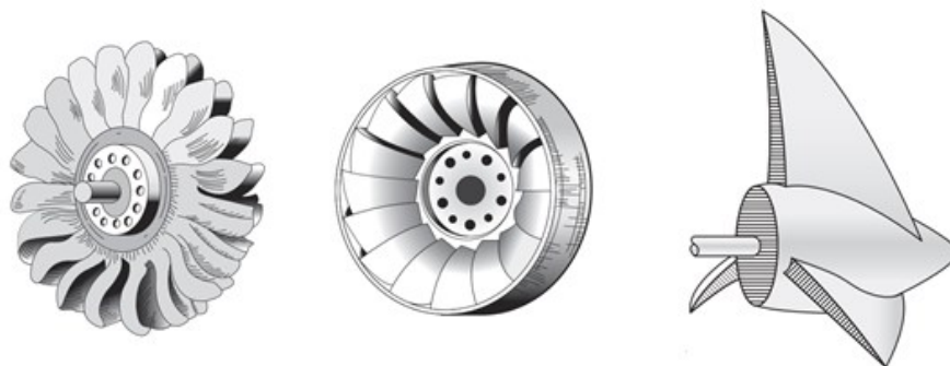
Figure 3. The most common hydropower turbines. From left to right: Pelton,
