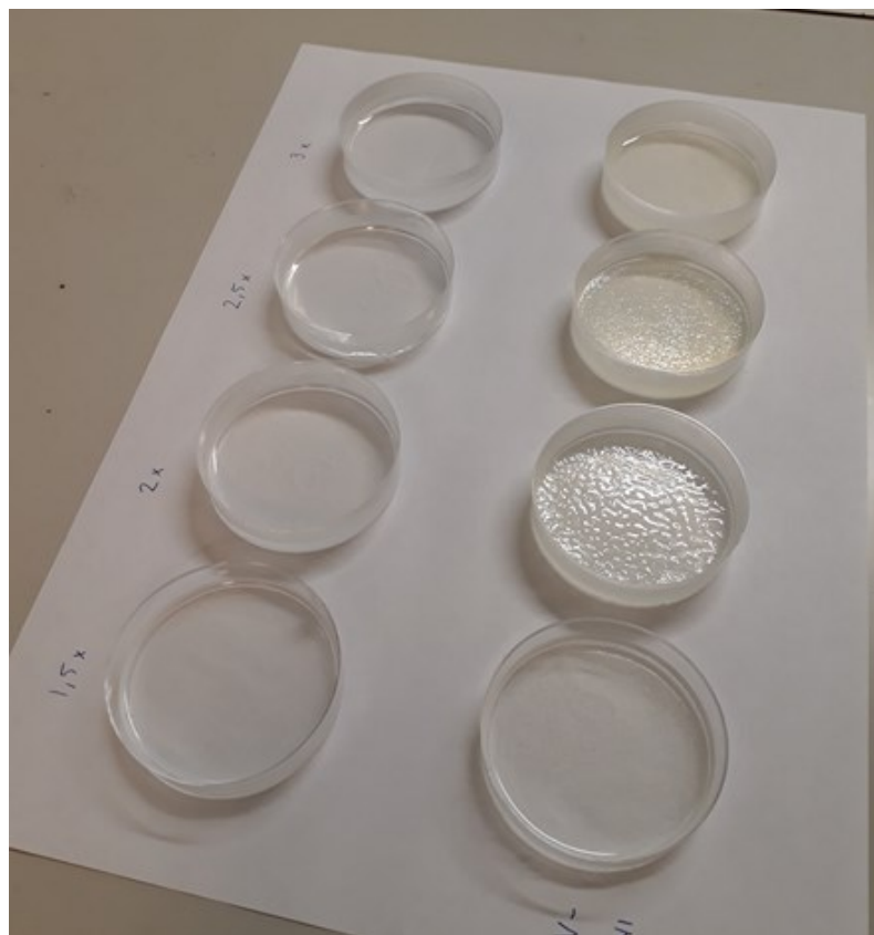
Figure 18. Gel samples prepared with photoinitiator or redox initiator.
