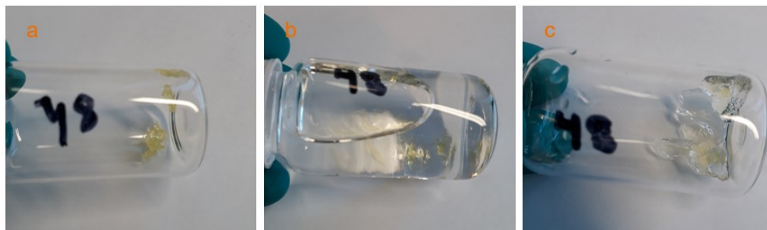
Figure 7. A dry gel (a), a partly swollen gel in water (b) and a swollen gel (c).
