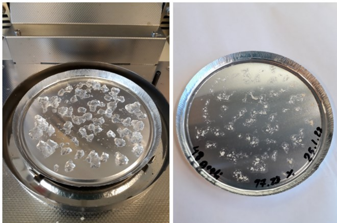
Figure 9. A gel sample before (left) and after (right) measuring the moisture content with IR-35 Infrared Moisture Analyzer (Denver Instrument).
