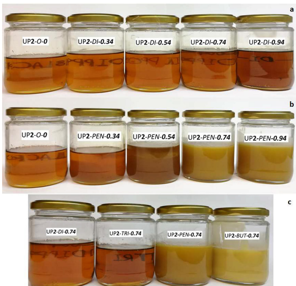
Figure 19. The appearance of samples made in two-stage: (a) di-PPG chain extended samples compared with the blank sample UP1-0-0; (b) pentanediol chain extended samples compared with the blank sample UP1-0-0; (c) samples with 0.74 molar ratio of different chain extenders.
