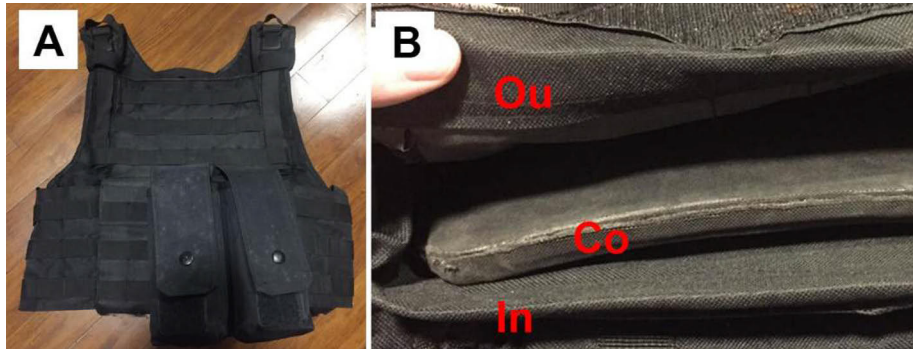
Figure 4.16. The design of a bulletproof vest (A), with the outer layer (Ou) and inner layer (In) made of kevlar and the core material (Co) made of steel, titanium, or bulletproof ceramics (B). Vest belong to Ganesh Aji Wicaksono, image was taken by himself and used with permission.
