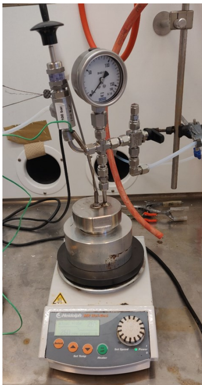
Figure 9. Autoclave for hydrothermal synthesis of (Co)-MoS 2 . During synthesis the autoclave was thermally insulated using insulation bandage.
