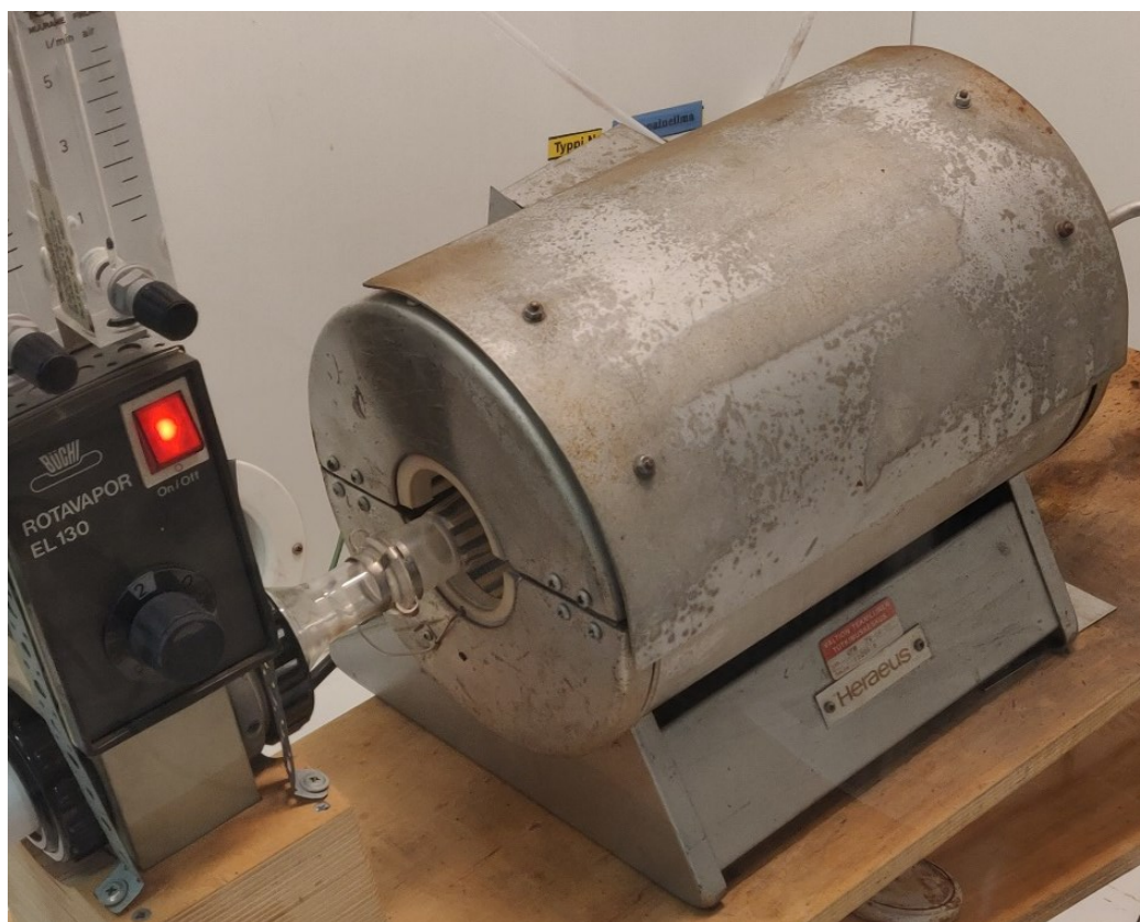
Figure 8. Rotating calcination oven used for calcination of prepared activated carbon catalysts.
