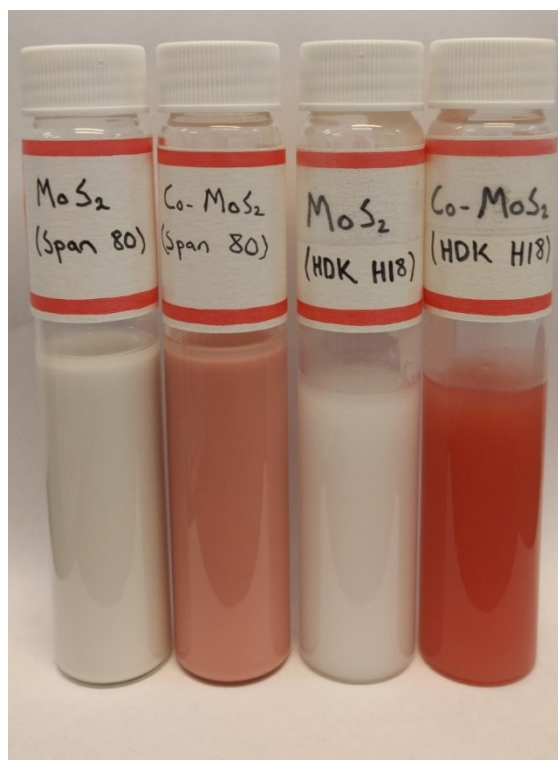
Figure 12. Side-by-side picture of prepared MoS 2 and Co-MoS 2 emulsion catalyst precursors using both Span 80 and HDK H18 surfactants.
