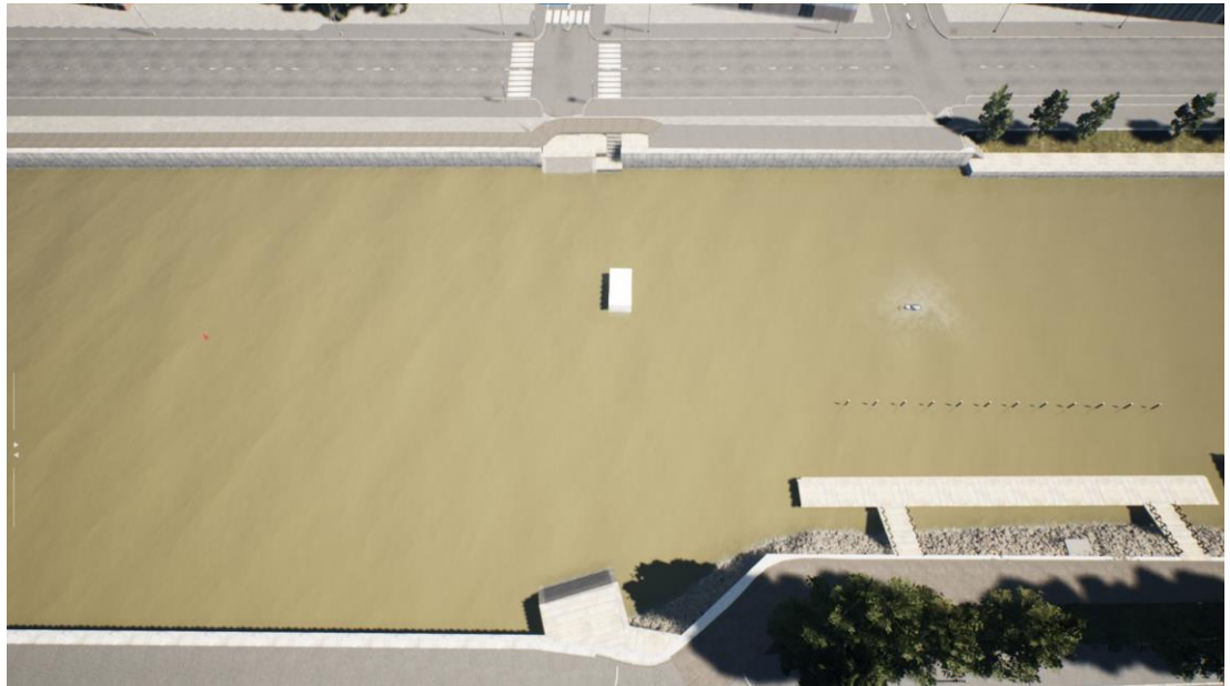
Figure 14. The more advanced scenario with moving obstacle in the middle, represented by a white cuboid. The controlled boat is on the left and the goals is to the right, represented by the red buoy.
