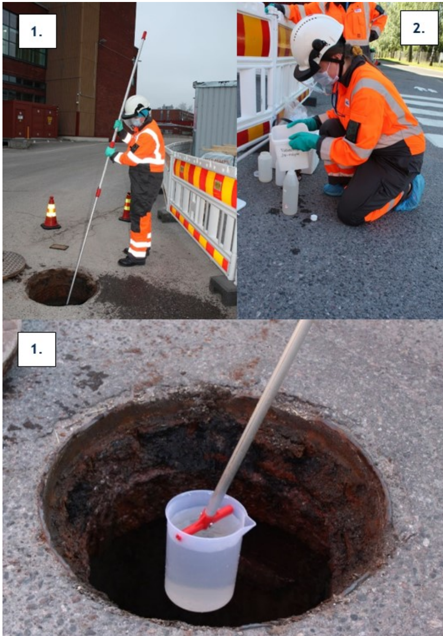
Figure 21. Sampling from the intermediate well. 1. Taking the process wastewater sample from the intermediate well and 2. Bottling the sample.
