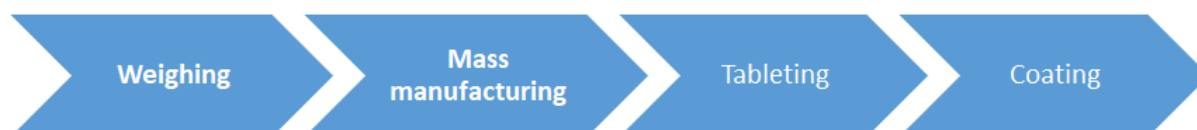
Figure 2. The unit processes of the tablet manufacturing processes. This study focuses on the weighing and mass manufacture unit processes.
