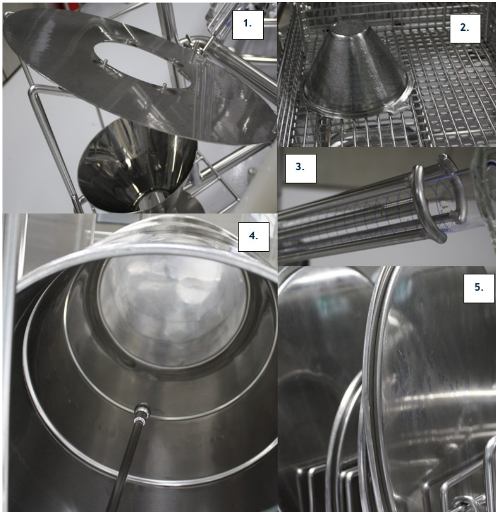
Figure 29. Equipment of the production line after pre-rinsing. 1. Mass container lid, 2. Sieve, 3. Measurement glass, 4. Vessel and 5. Lids of the vessels.
