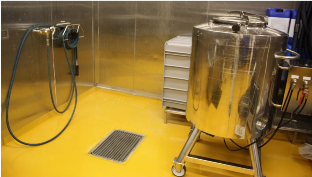
Figure 24. The rinsing area in the washing area of the mass manufacture process. Vessel of the granulation solution appears on the right side of the figure.
