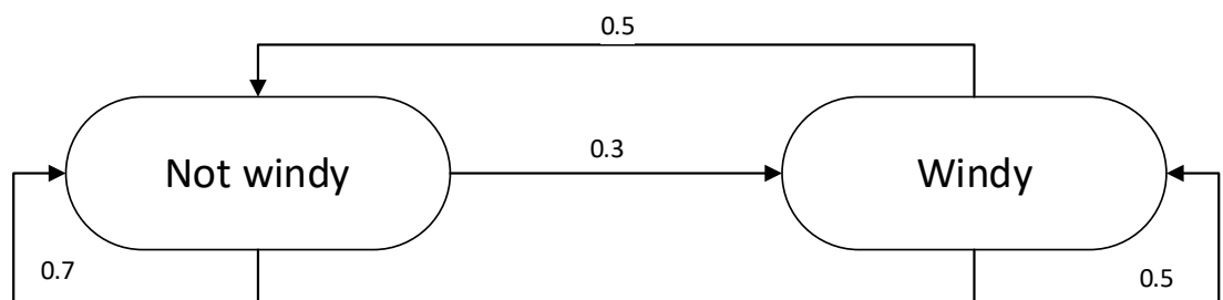
Figure 4. A picture of a Markov chain. In this example system, if it is not windy, there is a 70% chance of it remaining now windy and a 30% chance of it becoming windy. (Soni, 2018)
