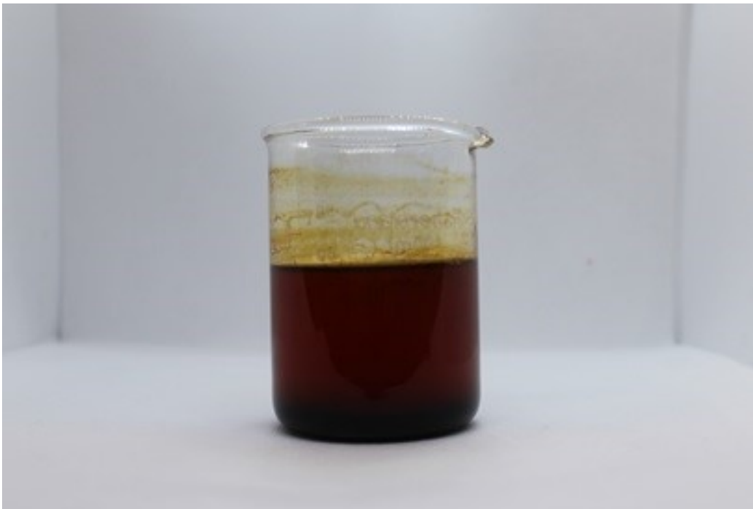
Figure 5.5. Lignin oil-Neste DMA emulsion with a mixture of surfactants TWEEN® 60 and Span® 80 (HLB 7.2) after 12 hours.
