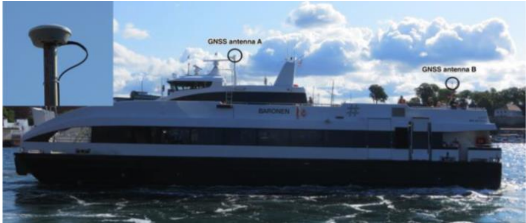
Figure 17. Baronen vessel including location of GNSS antennas /42/.
