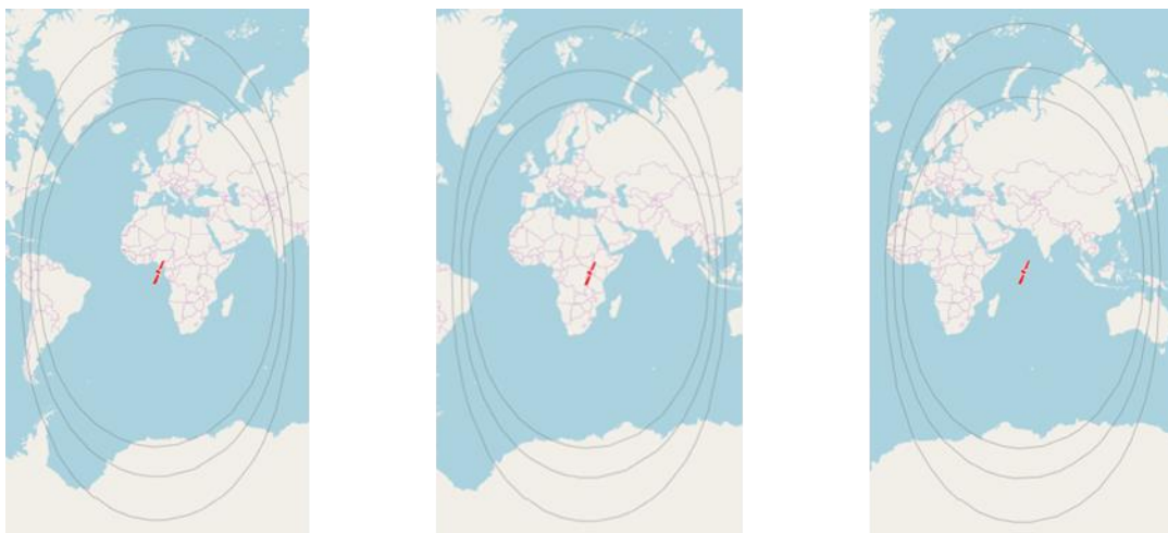
Figure 22. Locations and footprints of EGNOS GEO satellites PRN136 (left), PRN123 (middle) and PRN126 (right) /57/.
