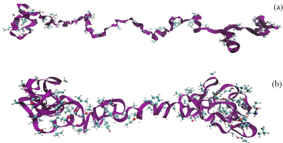
Figure 11 – Spring effect of flagelliform silk when subjected to stress and release a) extended state and b) relaxed state. In its extended state, intermolecular H-bonds that normally keep the structure crimped are broken. These sites have become free to bind (H-bond) with BC chains, resulting in strong adhesion between the two.
