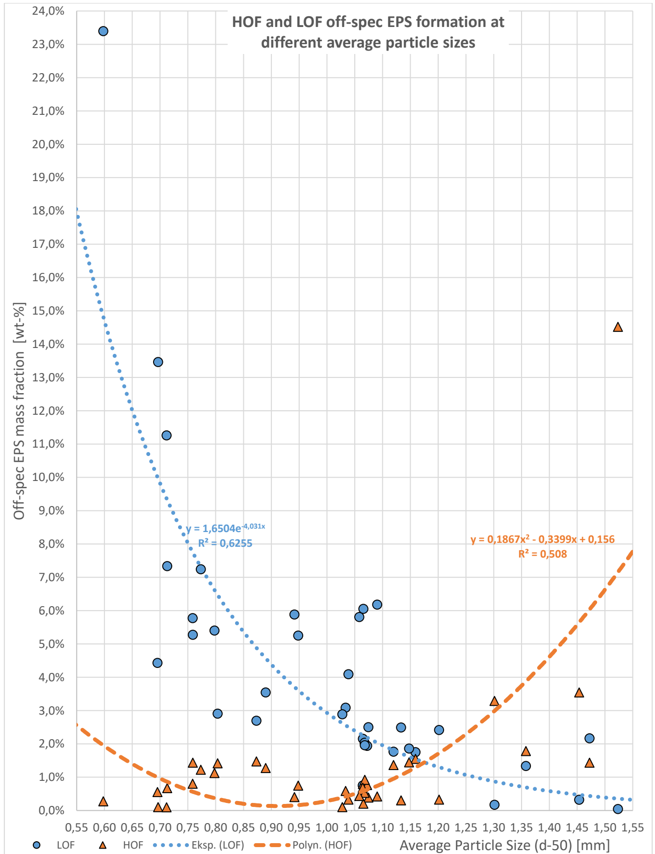
Figure 44. A collection of HOF and LOF EPS formation at different average particle sizes of all the samples.
