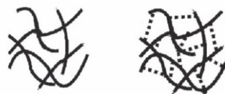
Figure 1. Thermoplastic (left) versus thermoset (right) [17].
