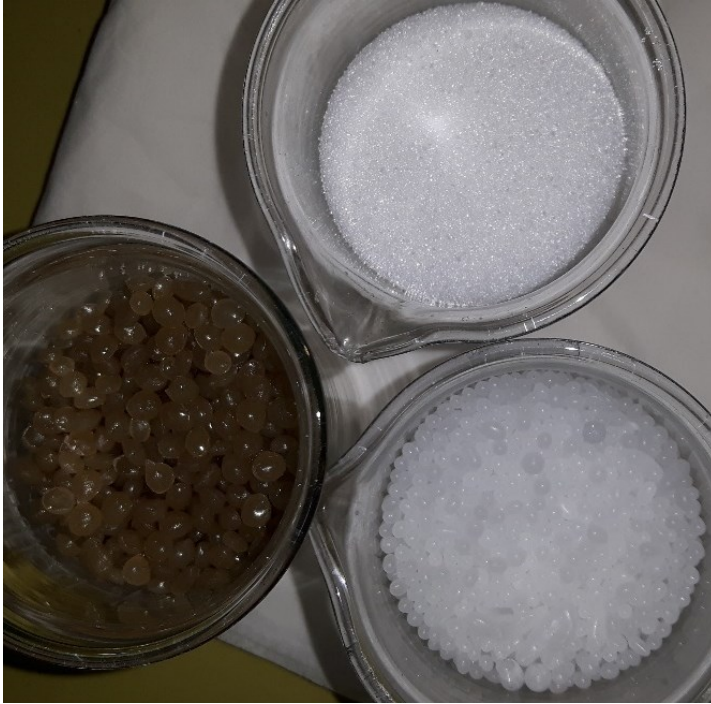
Picture 4. Raw materials used in polymerization and solubility experimentation (left bottom corner ERE, right upper corner LOF EPS [K-1310] and right bottom corner HOF EPS [K-110]).
