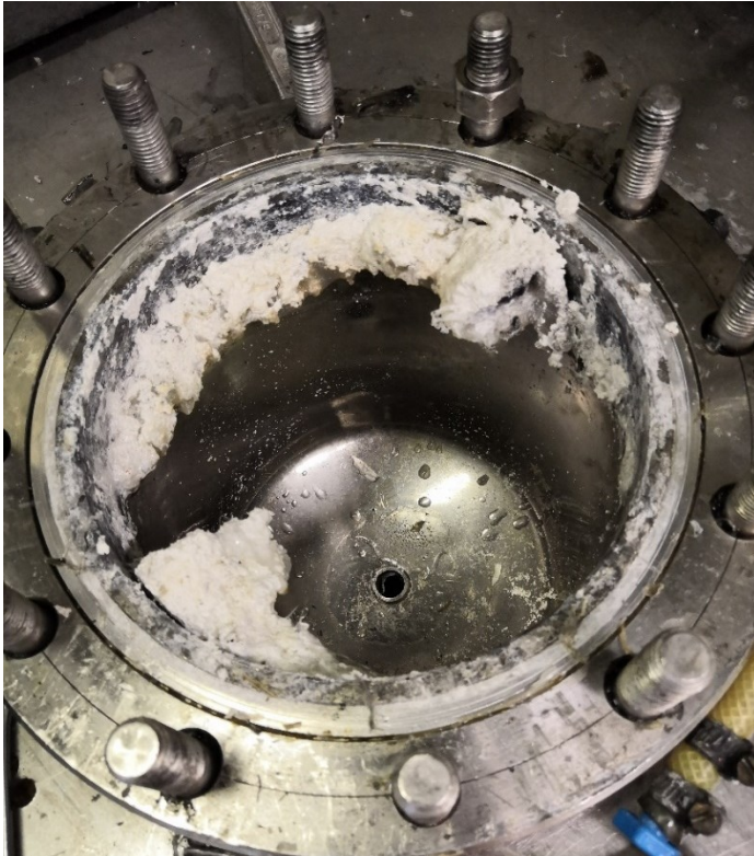
Picture 42. Picture of the reactor during purification when the lid was removed after preparation of 10 wt-% reused EPS containing batches, M-161.
