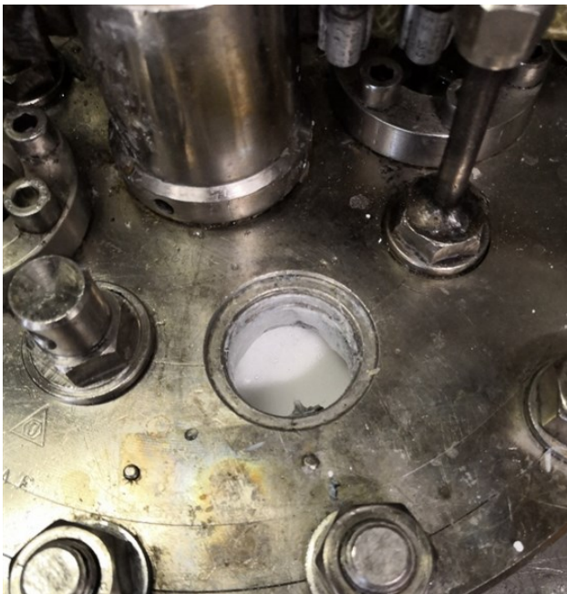
Picture 41. A picture of a foaming batch (10 wt-% K-1310 or LOF EPS, M-161).
