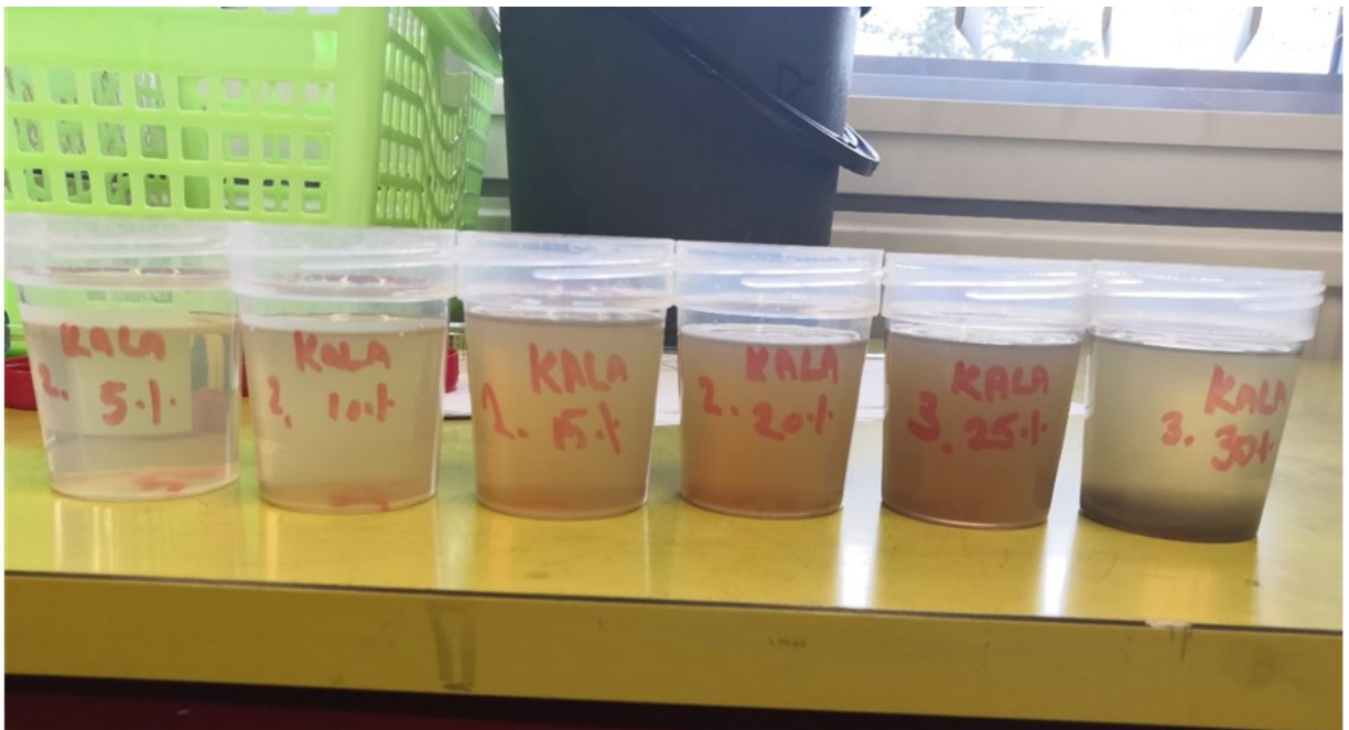
Picture 47. A picture of dissolved extruded recycled EPS (ERE) after weeks of storage with sedimentation (fish-box material).
