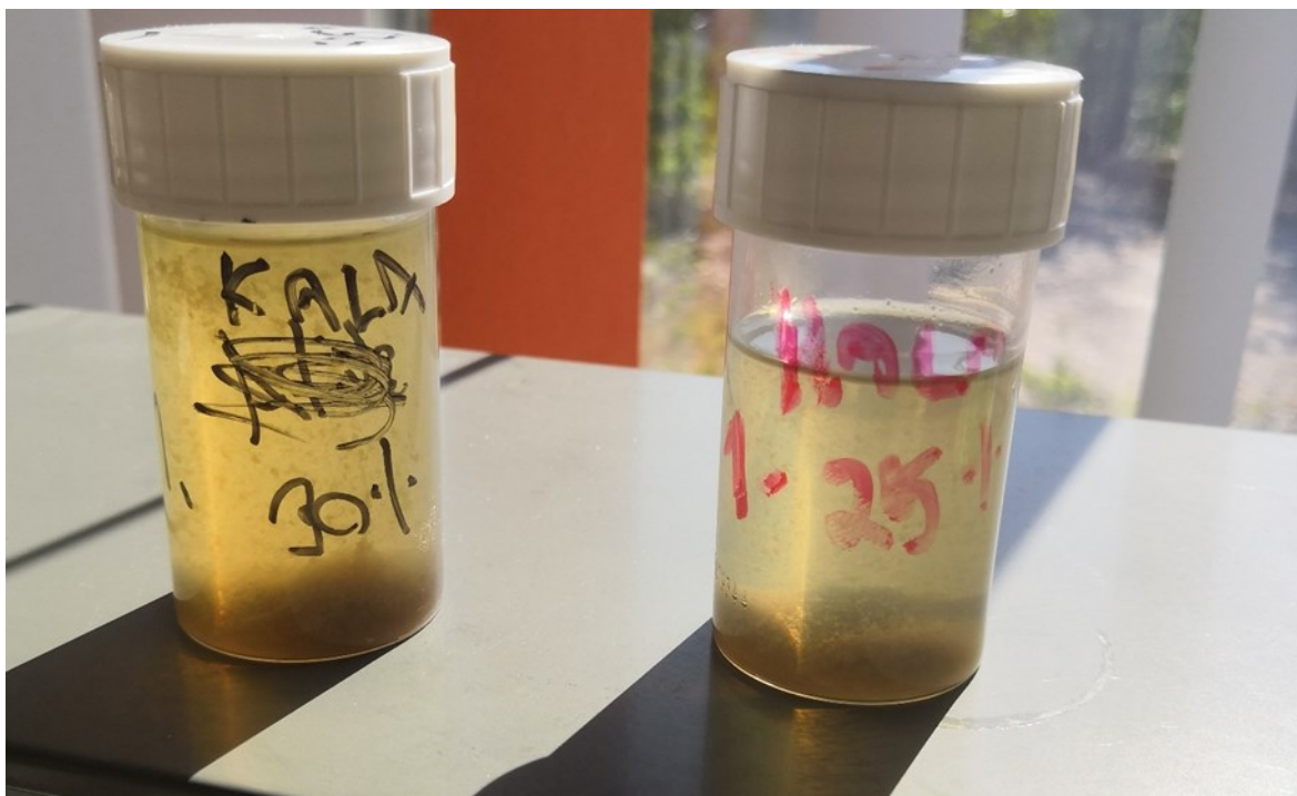
Picture 48. A picture of dissolved extruded recycled EPS after weeks of storage (fish-box material).
