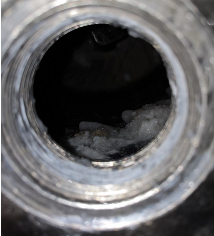
Picture 46. The M-reactor after the batch 14 % K-1310 or LOF EPS, M-165, with stabilization factor of 0.35 and stirring speed of 370 rpm (clusters and lumps on reactor walls and surfaces).
