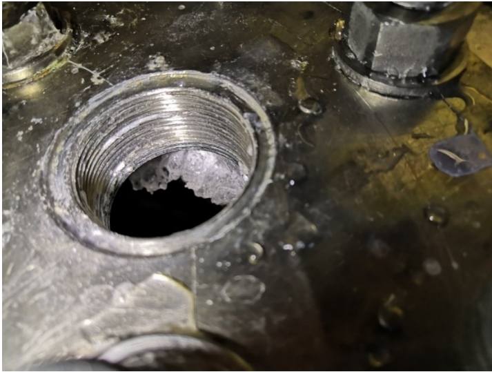
Picture 44. The M-reactor after the batch with 14 wt-% K-1310 or LOF EPS, M-166, with stabilization factor of 0.38 and stirring speed of 370 rpm (clusters and lumps on reactor walls).
