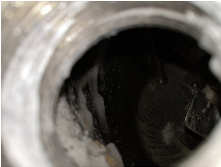
Picture 45. The M-reactor after the batch 14 % K-1310 or LOF EPS, M-165, with stabilization factor of 0.35 and stirring speed of 370 rpm (clusters and lumps on reactor walls and surfaces).
