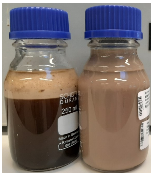
Figure 4.34 Dispersions polymerized with Stabilizer 3 and Initiator 1, at 85°C and pH 2.3 (left) and pH 5.0 with 40% more stabilizer (right). Clear phase separations were observed in the dispersion polymerized at pH 2.3 (left). Photo: Private.
