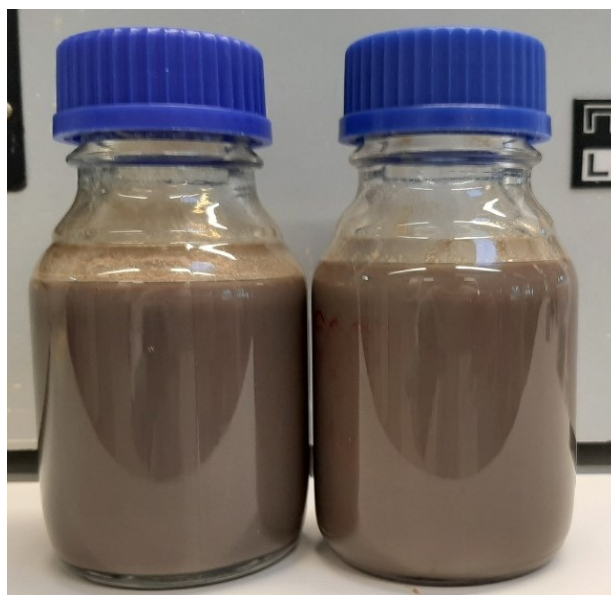
Figure 4.6 Dispersions polymerized with Stabilizer 2 and Initiator 1, at 85°C and at pH 5.0 (left) and pH 7.0 (right). No phase separation was observed, a small amount of dispersion was dried on the inside of the left bottle creating the illusion of a false phase separation. Photo: Private.
