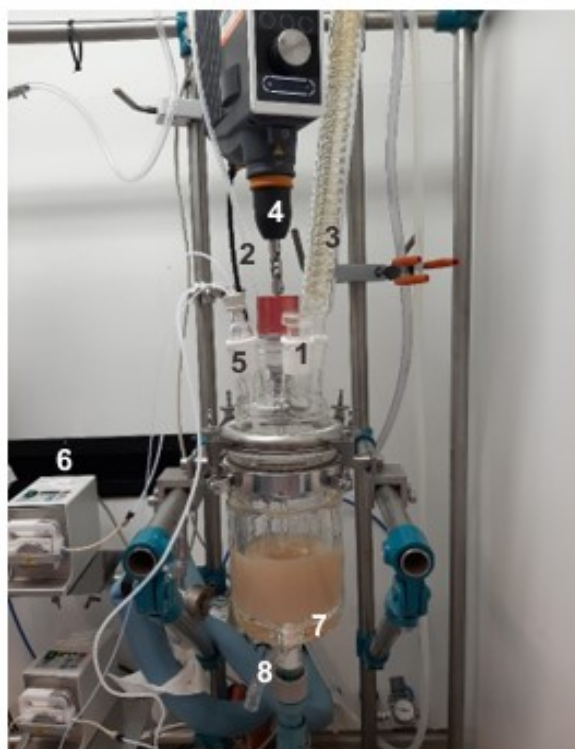
Figure 3.1 Scheme of the polymerization reactor and its functions, step 1 to 8. Photo: Private.
