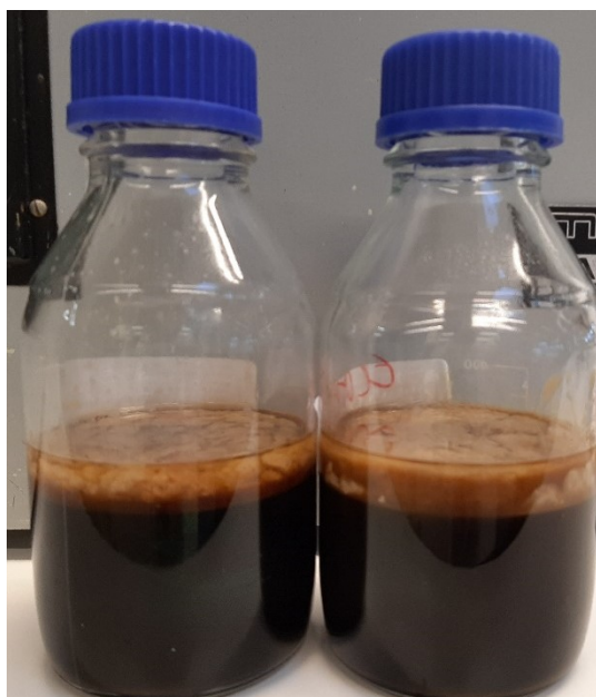
Figure 4.29 Dispersions polymerized with Stabilizer 2 and Initiator 2, at 85°C and pH 2.3 (left) and 5.5 (right). Clear phase separations were observed, indicating in unstable particles. Photo: Private.
