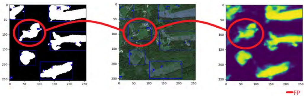
Figure 5.36: This prediction is fascinating because a significant false positive is detected. The system did not distinguish houses into the zone highlighted in red. The problem is that near the houses there is a damaged area and the algorithm has merged them.
