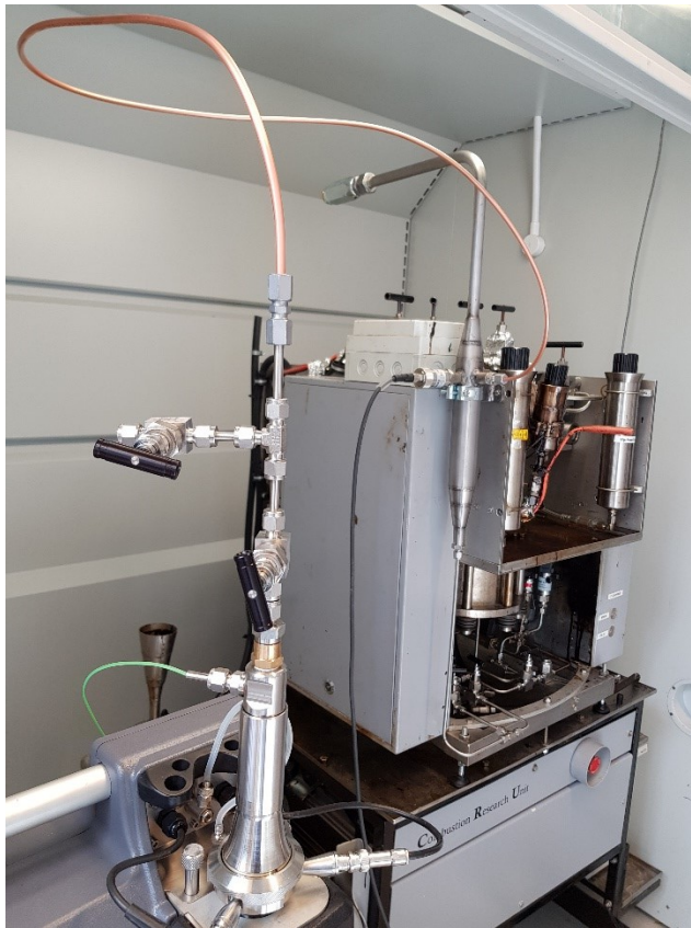
Figure 6. Setup version 2, with the installed copper duct connecting buffer tank B and ELPI.
