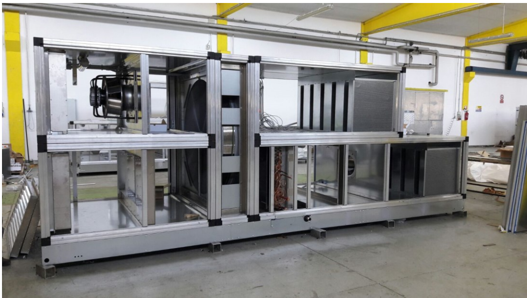
Figure 8: Air handling unit with enthalpy recovery wheel (Saiver)
