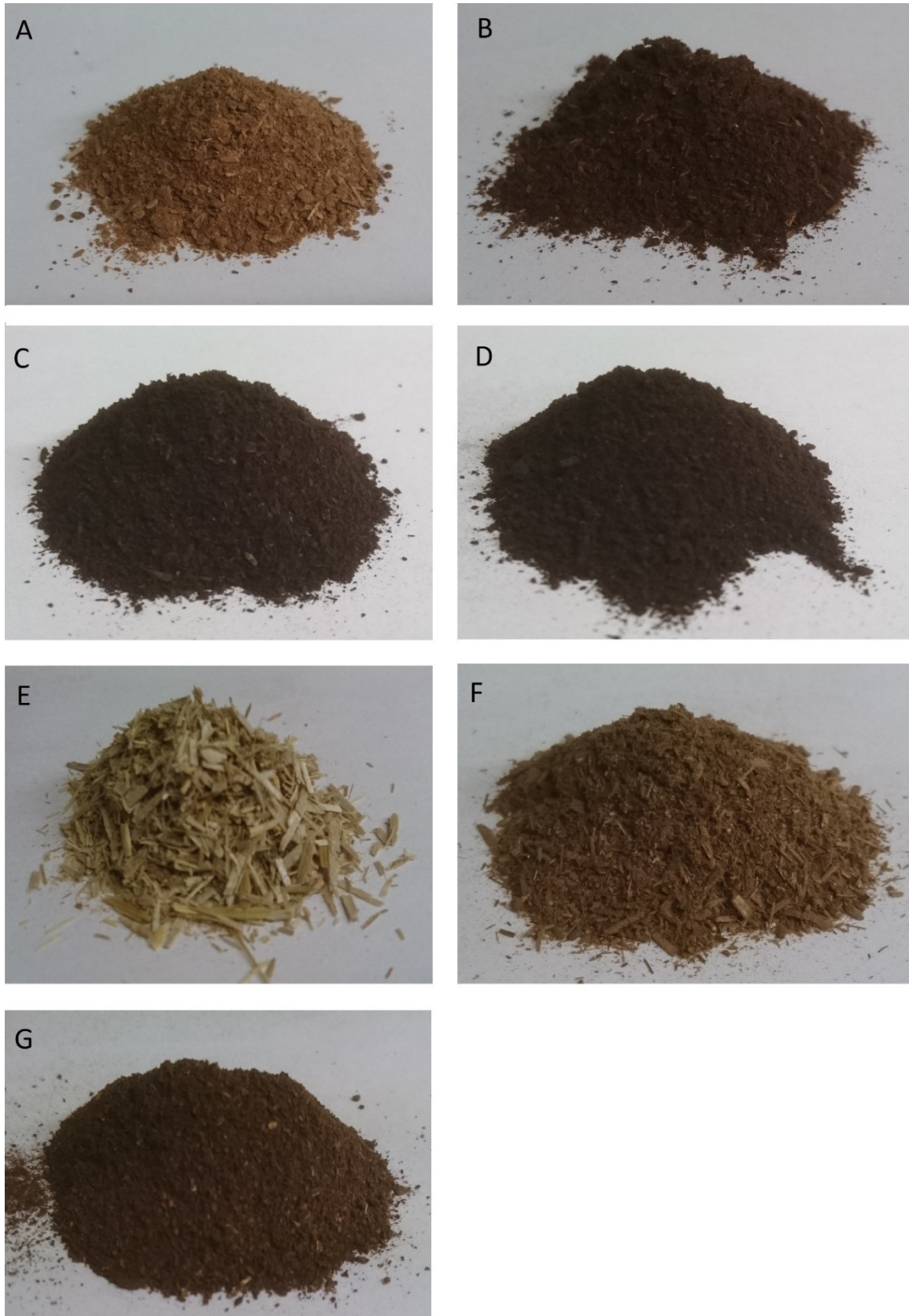
Fig. 5 Biomass samples after different pre-treatments; spruce bark (A), steam-exploded bark (B), torrefied bark (C), washed and torrefied bark (D), wheat straw (E), torrefied straw (F), washed and torrefied straw.
