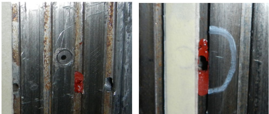
Figure 31 Installation of the pressure sensor on the cylinder surface
