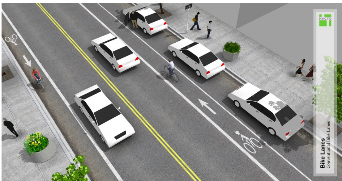
Figure 9 Two types of bike lanes. One next to parking, other without. (NACTO, 2014)
