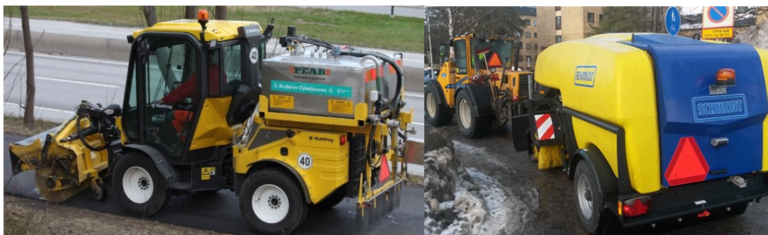
Figure 18 (left) Salt brush system on a single vehicle (Cykelpendla Hässelby, 2018)
