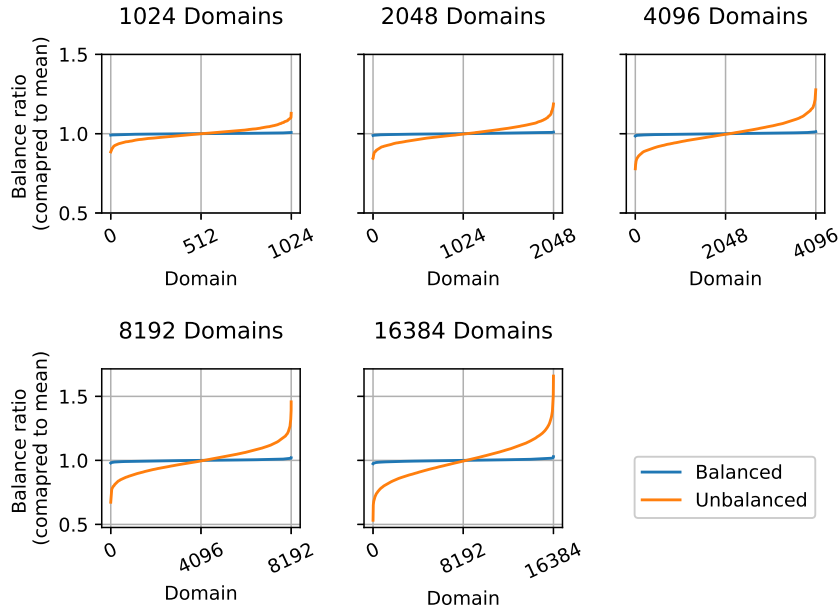
Figure 5.4: Illustration of the effect our load balancing has on the distribution of the fluid sites of the A4 sample, starting from 1024 subdomains and showing the distribution up to 16384 subdomains.
