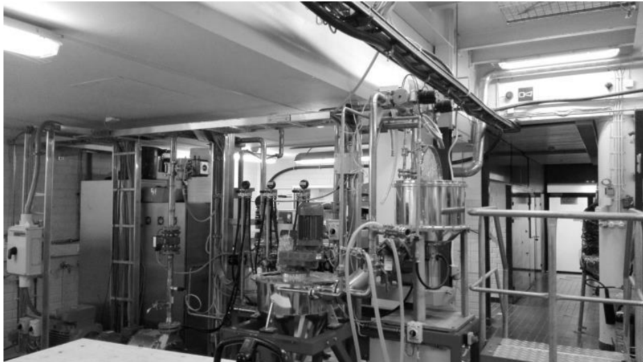
Figure 2.4 Image of low consistency refiner (ProLab).
