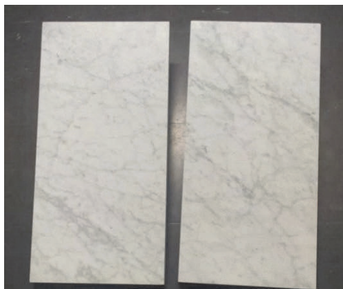
Figure 28. Untreated (left) marble and marble functionalized with Ma-24h-10% (right) produced for aesthetic evaluation.
