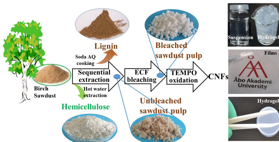
Figure 4. Scheme of the process to prepare CNFs from sawdust in a novel biorefinery concept.
