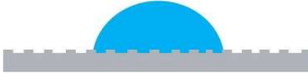
Figure 3. A liquid droplet in the Wenzel state.
