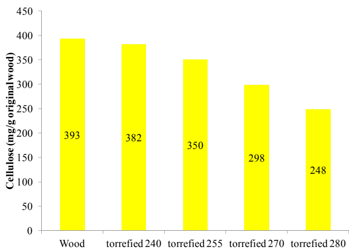
Figure 14. Cellulose content in birch and torrefied birch wood at different torrefaction temperatures (Paper II)
